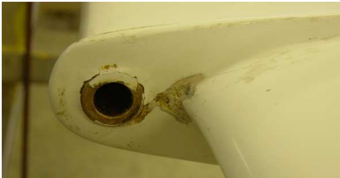
Possible form of damage to tailplane mounting node
